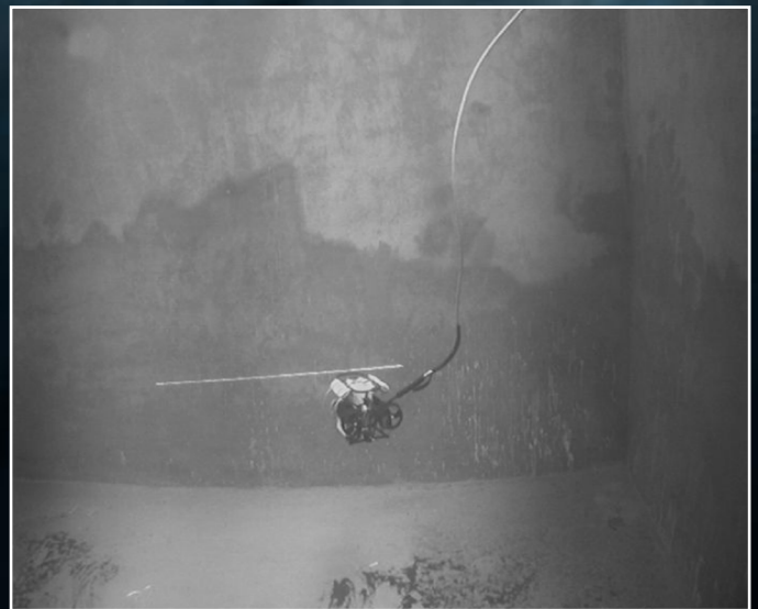
Micro-ROV equipped with Lumeneye VR horizontal profiler configuration
