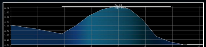
Measurements and profiles can be extracted from rendered laser model. Pipeline scar shown is 0.7mm deep and 8mm wide.
